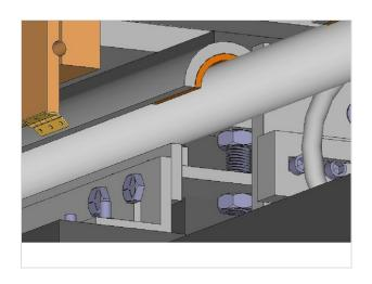
• The round ways are supported by a bar that is slightly off center so that there will be room for a carriage clamping device. Since a flat surface can only contact a round surface in a very small area, we take advantage of this fact by using just the edges of two flat surfaces to support the ways and to hold the carriage in place. Normally, cutting forces tend to press the carriage downwards but occasionally the clamps will be very necessary.
