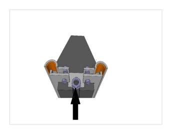
A long nut or handwheel should be added here.
