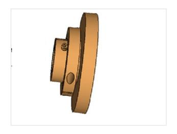
The chuck back plate (mount) is seemingly simple, but if you have to buy one it could cost more than the lathe itself! If you make your own, the two most common choices may be either a piece of cast iron that could be turned down to size or to make one from an aluminum casting. A cast aluminum back plate should have two clamp bolts and nuts (not tapped) on each side and an added steel safety collar. The hub will have to have a large enough diameter so that there will be clearance for the nuts.
