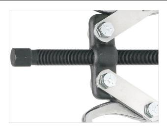
The cross slide lead screw could be a piece of threaded rod but parts from an old gear puller could work well since they usually have a fine thread and the screw is hardened. Later you could make a nut with a similar thread and use it with cupped washers to eliminate most end play.
