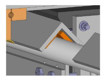
An angle iron alternative to the split pipe shoe. The brass wear strips could be eliminated if necessary.
