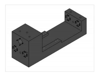
The concrete lathe "bed."
